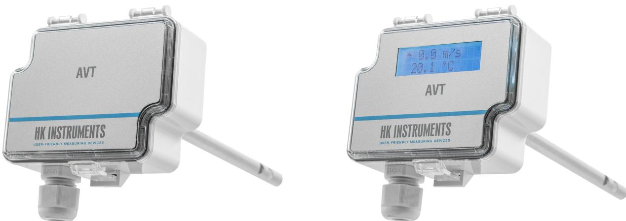
The AVT air velocity transmitters are electronic air velocity and temperature transmitters for air. They measure air velocity and temperature in ventilation ducts using a duct mount probe.
