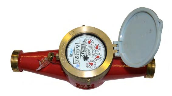
The VuAqua MJ-SDC-H is a multi-jet mechanical water meter with dry type dial counter suitable for a variety of metering applications including general purpose, sub-tenant and commercial metering tasks available in sizes DN15 (1/2") to DN50 (2").
