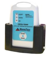
adgeTech's new ultra low temperature data recorder, records temperatures as low as -86°C. The Cryo-Temp can be used in a broad line of applications such as monitoring blood plasma, vaccines, pharmaceuticals, frozen foods and shipping containers. This stand-alone device does not require any additional probes. The enclosure is designed with a handle for
