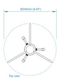
Positions for three off bolt fixings with Ø7.0mm (0.27") max. thread. on a p.c.d. of 85mm (3.35")
