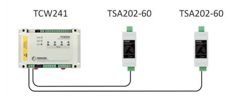
The "star" topology should only be used as a last resort, and only for up to 4 sensors with a maximum total cable length of 10 meters. Using a star topology may lead to increased signal interference and reduced communication reliability.
