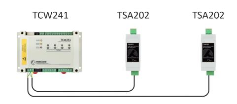
The "star" topology should only be used as a last resort, and only for up to 4 sensors with a maximum total cable length of 10 meters. Using a star topology may lead to increased signal interference and reduced communication reliability.
