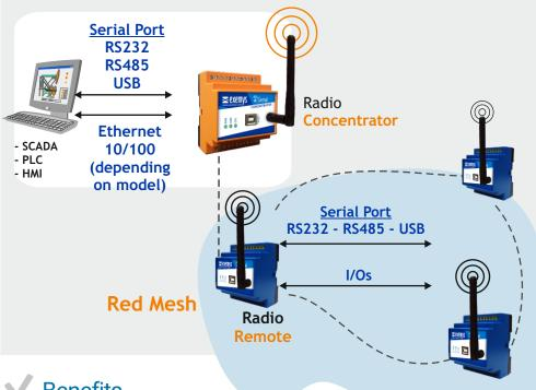
wSerial is a new concept in Serial Radio, which introduces Mesh Networks technology to achieve not only point to point, but also multiple connections.
