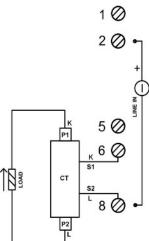
The input Voltage (LINE) has to be connected on terminals 2 (+) and 8 (as for the direct insertion).
