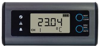
Monitor the environment you live and work in with the EasyLog EL-SIE-1. Configuration is simple, with no software to install on your PC or Mac – just connect the logger with a USB cable, and use your standard web browser to configure the device for logging. You don't even need internet access to set up and use the EL-SIE-1, it really couldn't be easier.
