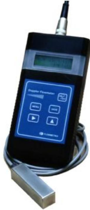
The Portable Doppler Flow Meter - PDFM3 is a handheld non-invasive microprocessor based meter for measuring the flow rate and total volume of liquids flowing through process and effluent pipelines. It is suitable for a wide range of liquids, including aerated water and liquids containing suspended solids, slurries and sludges. The PDFM3 requires fluids with a minimum concentration of 100 ppm of solids or bubbles having minimum size of 100 microns
