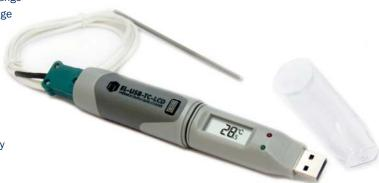
This standalone data logger measures and stores up to 32,510 temperature readings from either a K, J or T type thermocouple. A thermocouple is attached via the thermocouple socket at the base of the unit. The user can easily set up the logging rate and start-time, and download the stored data by plugging the data logger into a PC's USB port and running the purpose designed software under Windows 2000, XP, Vista or 7. Data can then be graphed, printed and exported to other applications.
