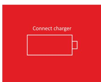
When the battery level is low, a warning screen (see left) will display for 5 seconds and the unit will power off.
