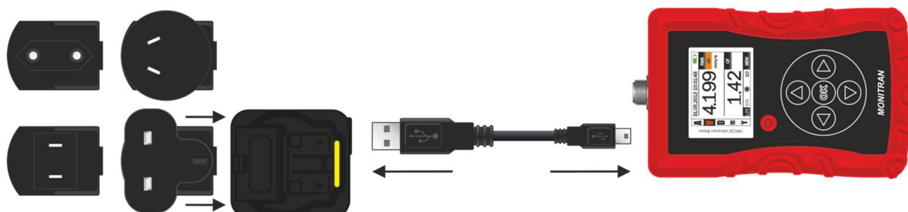
The unit should reach full charge within 4 hours. The battery status icon will indicate charging is in progress (see 6. Display & 8. Battery status).
