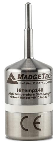
The HiTemp140 is a rugged, high precision, temperature data logger that is built for use in harsh environments. This stainless steel device is submersible and can withstand temperatures up to 140 °C (284 °F). With the HiTemp140's standard calibration, an accuracy of +/-0.1 °C (0.18 °F) can be achieved over a wide temperature range.
