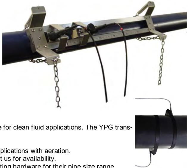
WPG, XPG, YPG and YPGD transducers operate in transit time mode and are for clean fluid applications. The YPG transducers are especially good with lined pipes\* and applications above 100mm.
