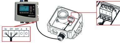
Wiring in parallel of 2 OLCT 10 detecting same gas (CO, NO or NO<sub>2</sub>)
