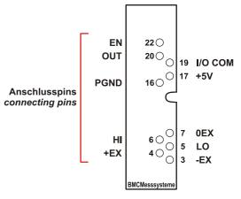
The pin assignment of the MA-U corresponds to the 5B modules of Analog Devices and Burr Brown. An additional 0EX pin (pin 7) has been introduced as reference for +EX and -EX. If using a non-bmcm backplane that does not provide a relating connection, this pin has to be removed. Then, however, a reference of the  $\pm$ EX pins is only possible via the LO pin with J7 being closed. This is a specific assignment of BMC Messsysteme GmbH. The 0EX pin is not connected in modules of other manufacturers.
