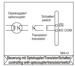
The output switch and EN have a reference to I/O COM. If the EN control signal is referred to PGND, a high-ohmic connection (e.g.  $10k\Omega$ ) must be made between I/O COM and PGND (This influences the galvanic isolation between PGND and I/O COM!).
