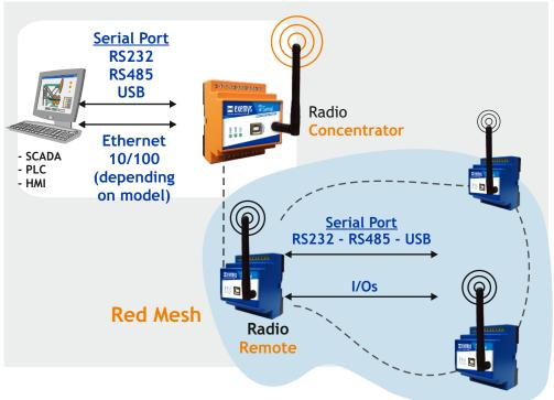
wSerial is a new concept in Serial Radio, which introduces Mesh Networks technology to achieve not only point to point, but also multiple connections.
