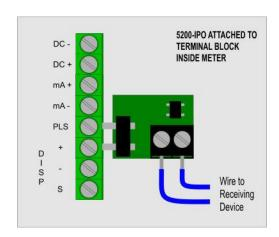
The pulse output built into CDI flowmeters is an opencollector transistor output that functions as a switch to the meter's ground. It does not provide electrical isolation between the meter and the receiving device. The IPO provides this isolation.
