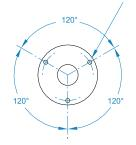
Pipe Mount 34 mm (1.34 in) diameter (standard 1 inch pipe) option with Terminal Strip Junction Box
