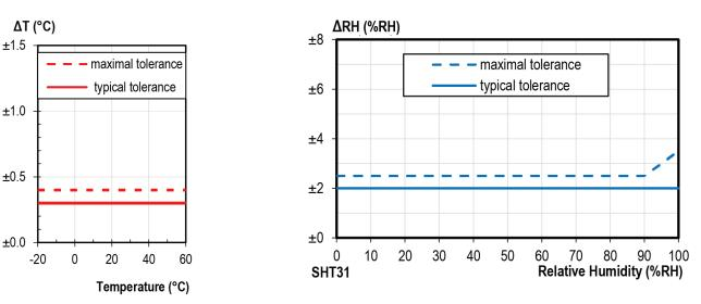
Typical and maximal tolerance for the temperature sensor in °C: Typical and maximal tolerance for the relative humidity sensor at 25°C:
