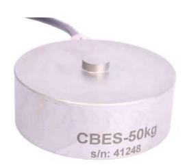
The CBES series of low profile button load cells are designed for the measurement of compressive forces. Its compact size and low height means it can be used in applications where height is at a premium and is often retrofitted. It is suited for both force measurement and weighing applications such as vessel weight measurement. Special customisation options are available and include IP68 rating for fully submersible applications, please speak to our sales team.
