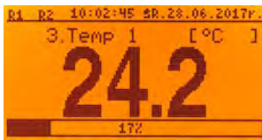
Real time measurement value 18 mm high digits
