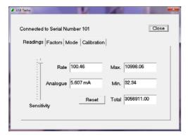
In use the device will operate as a stand-alone module. However, by connecting to the USB port, users can access an on-screen display that shows current operational status and the input sensitivity setting.
