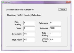
All required operational parameters, such as scaling factor, high and low alarms, etc., are entered via onscreen dialogue boxes, and once entered are stored in non-volatile memory.
