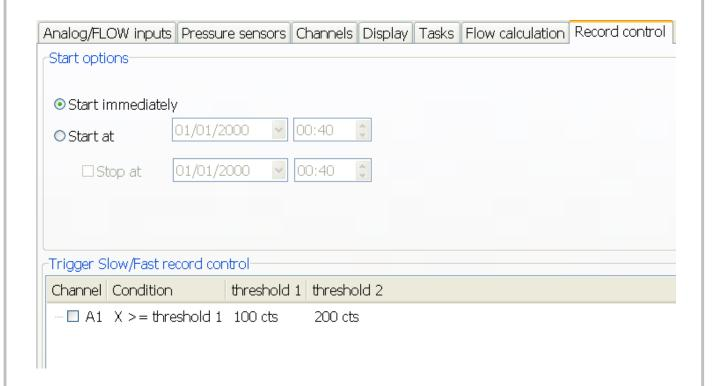
Once the setup has been completed it can be saved and uploaded to the data logger. Configurations can also be downloaded from the logger, modified, saved and uploaded back to the logger.
