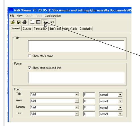
The setup for the graph including X and Y axis, curve colours and thickness can be accessed in setting menu.
