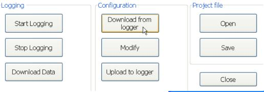
You can download the configuration that is in the logger by clicking on the Download from loggerg button. Once it has been downloaded you can modify the program by clicking on the Modifygor you can open an existing project saved on the PC by clicking on the **D**pengbutton.
