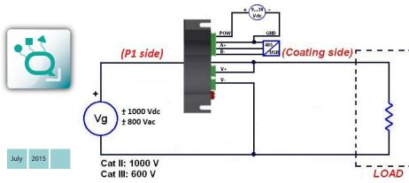
CAUTION: Magnetic fields of high intensity can vary the values measured by the transformer. Avoid installation near permanent magnets, electromagnets or iron masses that induce strong changes in the magnetic field. If any irregularity recommend reorient or move the transformer in the area most appropriate.
