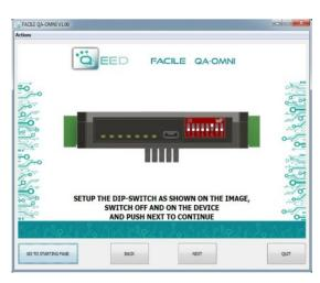
It is possible to use the program without connecting to the module, in this mode you can SAVE the configuration on your PC, which can then be sent to the OA-OMNI at a later time.
