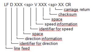
The checksum is all information in the string added, the least significant byte is divided into high and low nibble and both nibbles are incremented by hexadecimal 30. This information is sent out as a checksum.
