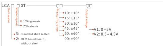
E.g: LCA310T-10-v1: Single-axis/Standard /±10°Measuring range/0-5V output voltage
