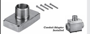
The Conduit Adapter allows you to enclose wiring from the magnetic pickup. The kit includes a turbine meter cover with a 1 inch male NPT conduit fitting and screws for plastic or metal installation.
