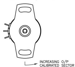
SHAFT FLAT ALIGNED WITH MOUNTING SLOT AT MID TRAVEL ±5°.
