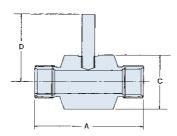
Allow an extra 50 mm height on dimension 'D' for pick off coil connector.
