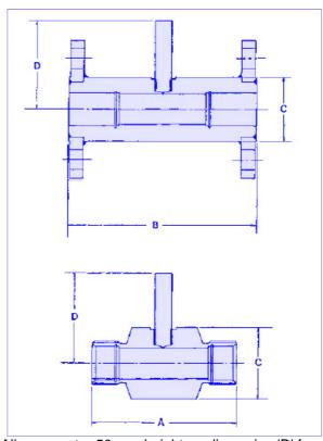
Allow an extra 50 mm height on dimension 'D' for pick off coil connector.
