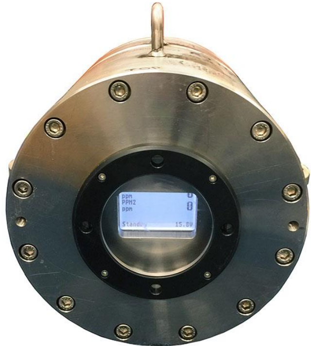
Merlin Logger fitted in a large housing suitable for up to 12 external sensors
