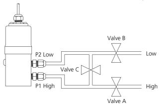
Valve A = High side valve Valve B = Low side valve Valve C = Shunt (bypass) valve
