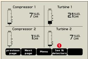
1 Up to 16 detectors can be displayed simultaneously
