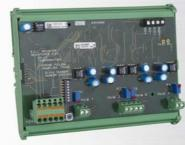
Addressable 4- analogoutput module which delivers 4 analog 4-20mA signal outputs (detector output copy, min, max, average of a group of detectors) for connection to a datalogger, a PLC, a Building Management System (BMS), etc.
