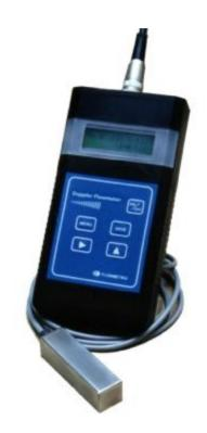
The Portable Doppler Flow Meter - PDFM3 is a handheld non-invasive microprocessor based meter for measuring the flow rate and total volume of liquids flowing through process and effluent pipelines. It is suitable for a wide range of liquids, including aerated water and liquids containing suspended solids, slurries and sludges. The PDFM3 requires fluids with a minimum concentration of 100 ppm of solids or bubbles having minimum size of 100 microns
