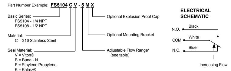
\* Adjustable Flow Rate Set Point Nitrogen @ 5 psig (0.34 bar)
