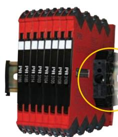
**Installation on a 35 mm DIN rail**
