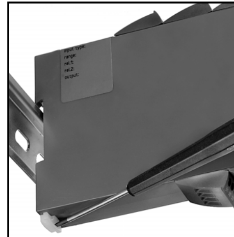
Picture 1: Separation from DIN rail.
