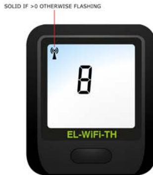
4) RECEIVED SIGNAL STRENGTH INDICATOR (RSSI) (VALUE BETWEEN 0 & 10)
