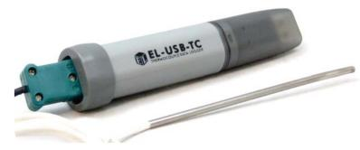
This standalone data logger measures and stores up to 32,510 temperature readings from either a J, K or T type thermocouple . A thermocouple is attached via
