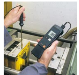
Surface temperature in moulding tools
