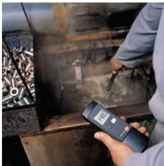
Measures temperature in oils e.g. in burnishing vats
