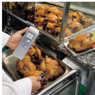
Measures core temperature of chickens, for example, just prior to being served
