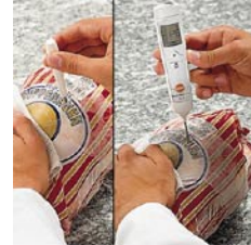
Measures core temperature in deep-frozen products: first drill, then measure
