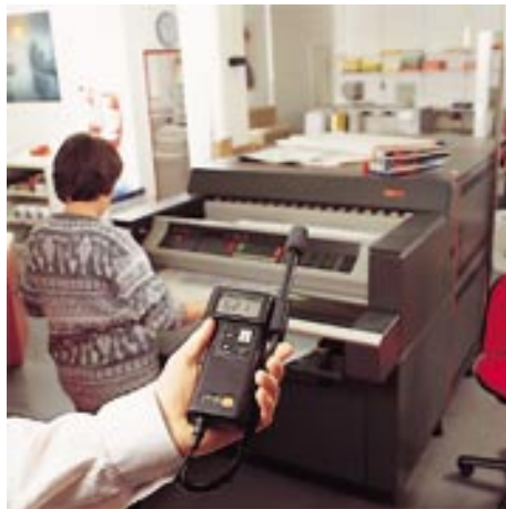
Measures office noise e.g. photocopiers, printers etc., accuracy class 3
