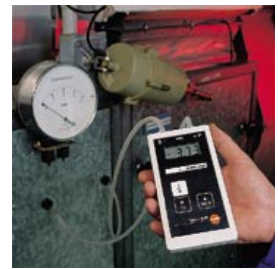
Measures differential pressures across air filters (checking a manometer)
