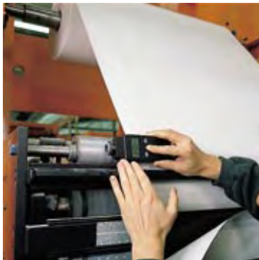
Mechanical rpm measurement on a roller
