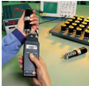
rpm measurement in a reduced d.c. motor
